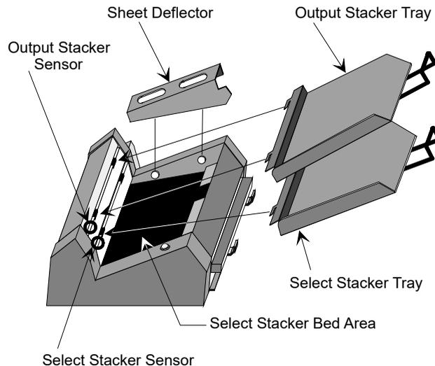
Errors are generally caused by either paper or debris that block the output or select stacker sensors. In most cases, clearing the paper jam or cleaning the sensors will resolve the issue.
