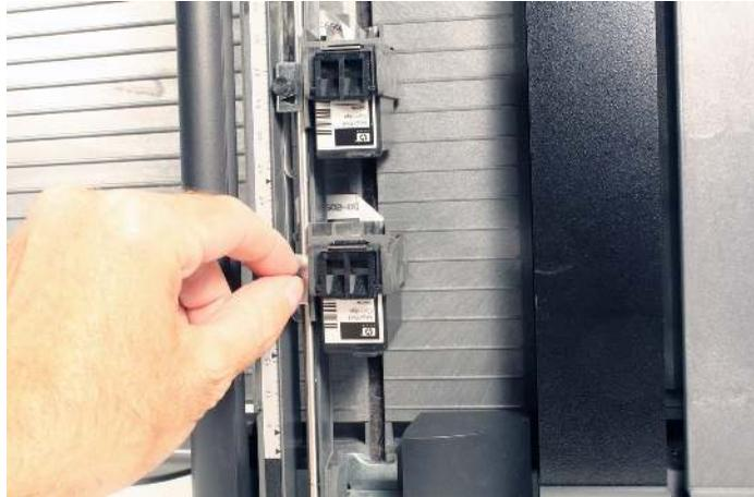
5. Adjust the position of the second printer to the 6.2 inch mark.
