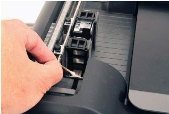
**CAUTION:** Do not spray any substance directly into or on the cartridge holder.
