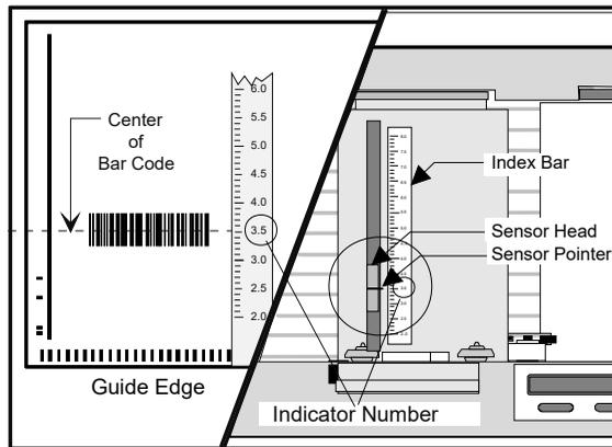
3. Check the scan path on the sheet. Make sure that there are no stray marks, black marks or printing in the scan path that leads to or from the bar code.
