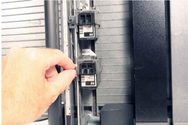
6. Move the printer to the desired position and lightly tighten the thumbscrew.
