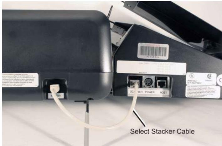
6. Plug in the Select Stacker by performing the following. Connect the power cord to the power strip. Connect the power supply to the power cord. Finally, connect the power cable to the Select Stacker as shown. It is acceptable to plug the Select Stacker, the scanner, and the host computer into the same power strip.
