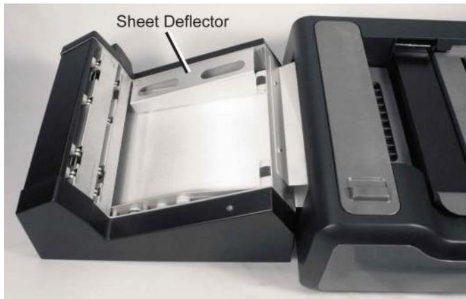
3. Mount the select stacker (lower) tray to the Select Stacker. The metal hooks go into the slots in the Select Stacker.
