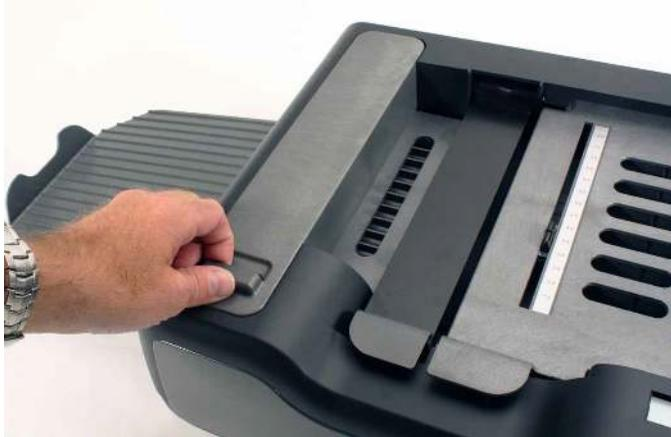
2. Remove the cartridge by holding the printer cartridge tab and pivoting the used cartridge out of the cartridge holder.
