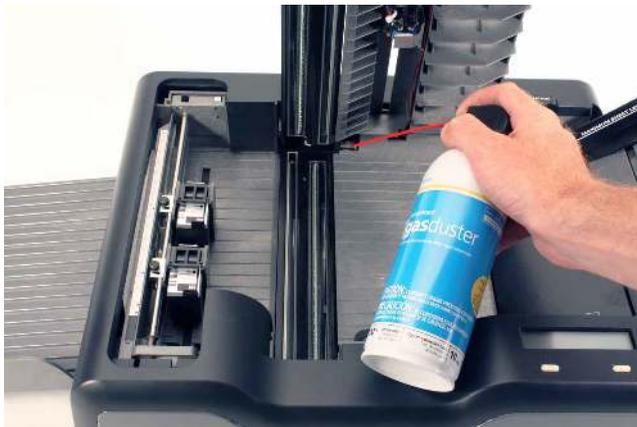
**CAUTION:** Do not use the canned air after this step as it can blow dust on areas that have been cleaned.
