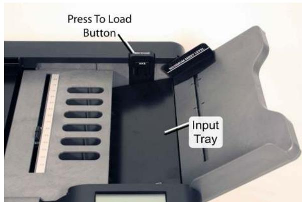
4. (Optional) If you have a large number of sheets to load, you may want to secure the Press To Load button in the down position by pushing in the **Tray Lock** while the button is depressed. To release the lock after you have loaded sheets, depress the **Press To Load** button once again and release it.
