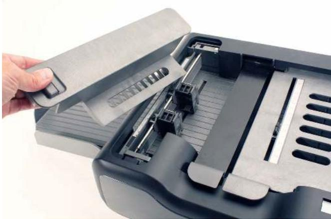
2. Notice the location of the cartridge holder that is inside the printer assembly. Also notice the ruler, the printer alignment mark, and the thumbscrew that sit beside the cartridge holder. These are the elements used to position the printer(s).
