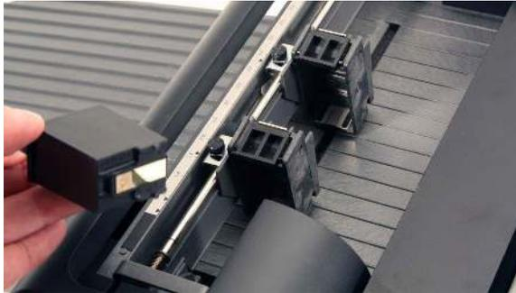
3. Using a clean swab, gently wipe the area of the cartridge holder that contains the electrical contacts.
